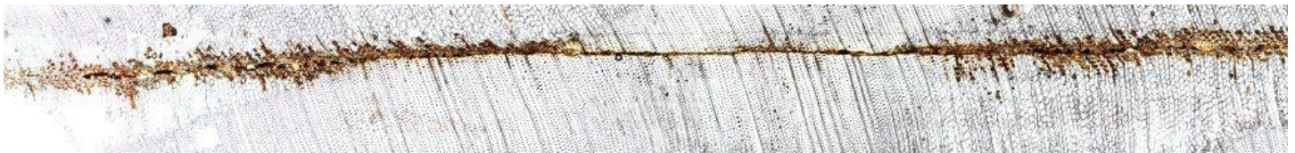
Entire bondline image, unstained, southern yellow pine, phenolic adhesive, brightfield, K. Mirabile
