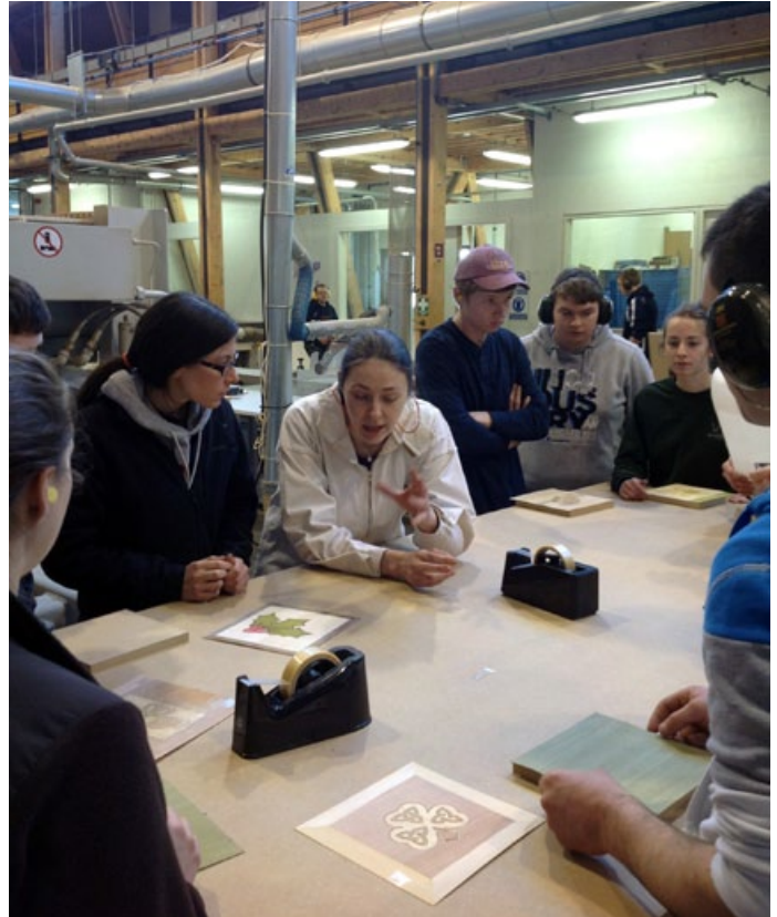
Galway-Mayo Institute of Technology Instructor Ann Foley (center) explains the marquetry veneering process to Virginia Tech student Zoe Carroll (left) and other students. Virginia Tech students designed and produced the marquetry to represent their impressions and experiences in Ireland.
