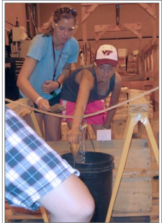
YCC students see how much a piece of wood will bend before it breaks.
