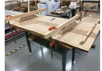
“Problem Child” fitted with stabilizing cross members to remove warp.
