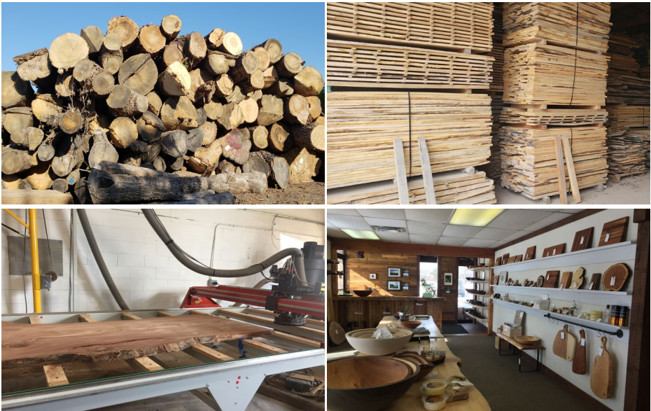
Figure 16. Stages of urban wood utilization. Clockwise from top left: urban wood logs, kiln-dried lumber sourced from urban logs, surfacing machine commonly used for live-edge boards, finished products. Photo credits: Omar Espinoza, Anna Pitti.
