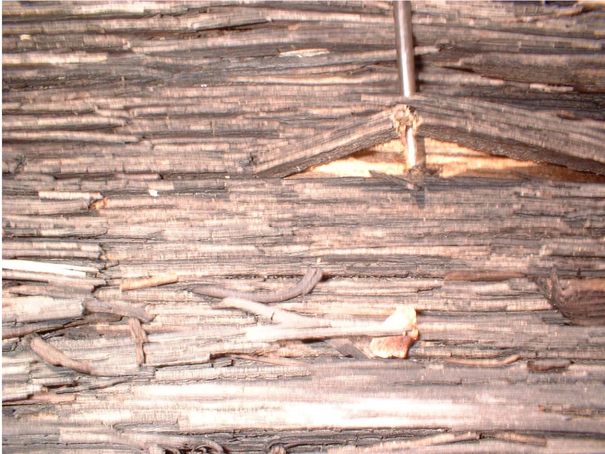
Figure 1b. This decayed wood broke easily. The break occurs across the grain without splintering.
