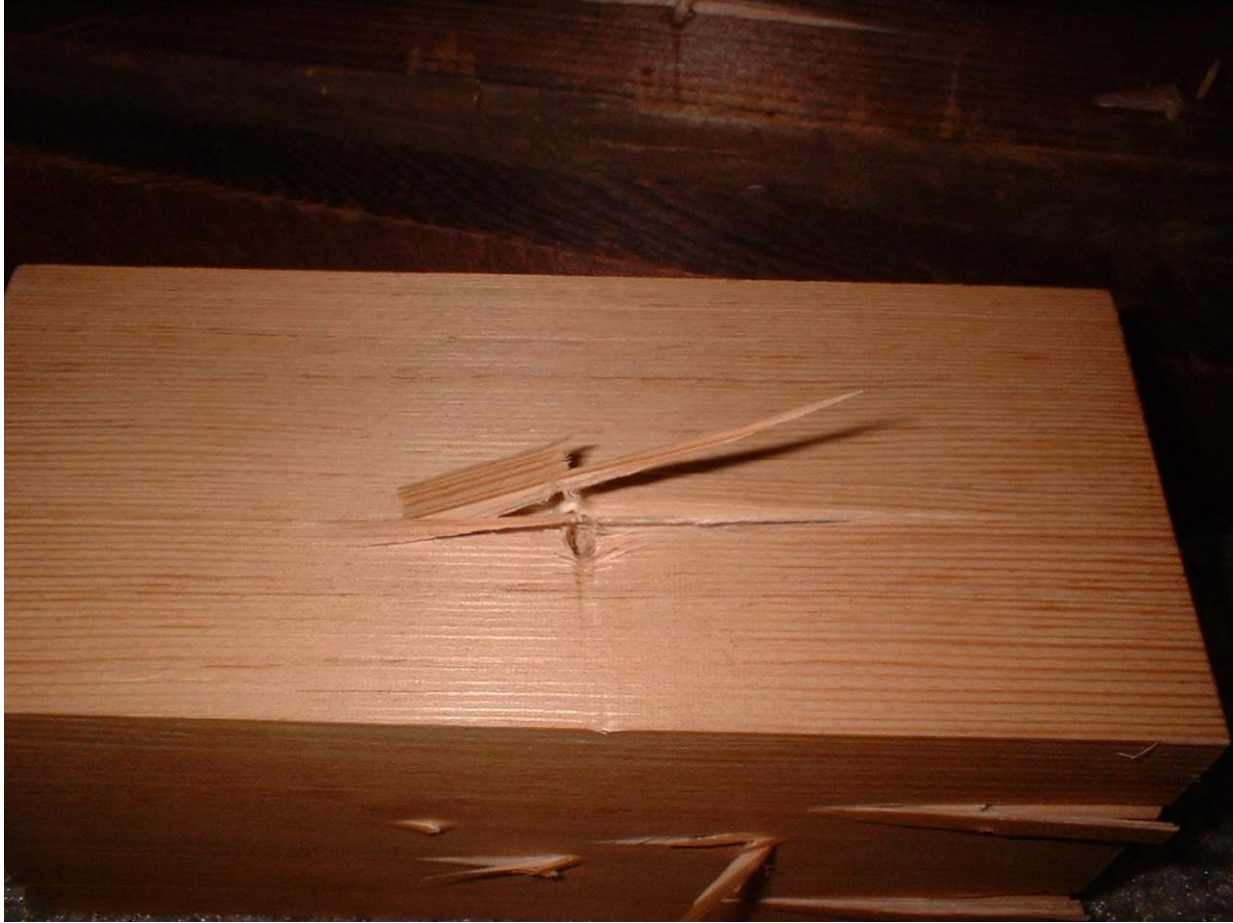
Figure 2. This sample is a block of virgin Douglas Fir with no decay. It shows a splintered break that begins far from the penetration.
