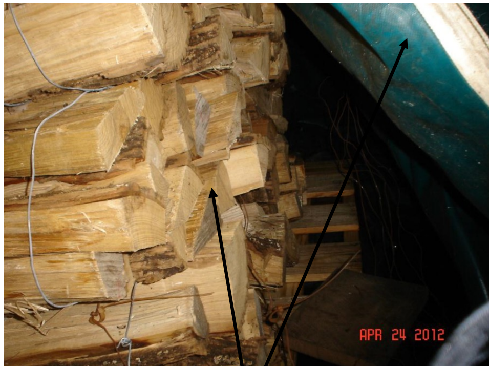
Firewood bundles in flexible steam/vacuum chamber
