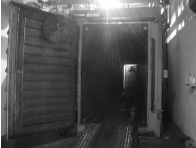
Chamber: 6 ftX9ftX64ft long, pre-heated walls
