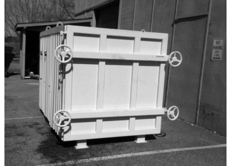
5X5X8.5 foot vacuum chamber
